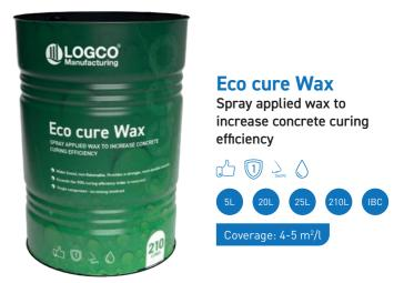
Eco cure Wax is a white, water based low viscosity wax emulsion, which when spray applied to the surface of fresh concrete forms a clear film on drying. eco-cure wax will greatly increase concrete curing efficiency, by retaining moisture, enhancing cement hydration thus providing a stronger, more durable concrete. Suitable for all concreting particularly for large areas, floors & carriageways. Will greatly increase concrete curing efficiency above 90%.
