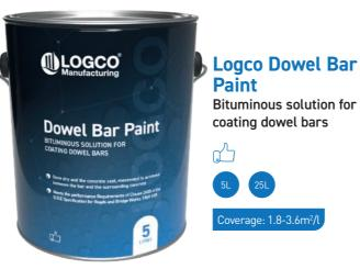
Logco Dowel Bar Paint is a bituminous solution designed to provide a thick film on dowel bars. Once dry and the concrete cast, movement is achieved between the bar and the surrounding concrete. It meets the performance Requirements of Clause 2605 of the D.O.E Specification for Roads and Bridge Works 1969 109.
