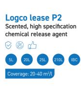
Logco lease P2 is an extremely versatile high class chemical release agent blended with highly active surfactants. The blend of highly active surfactants assist in reducing surface tension at the interface between the concrete and the formwork. Thus ensuring that optimum release is attained hence achieving a high quality concrete surface finish. With added pine fragrance.
